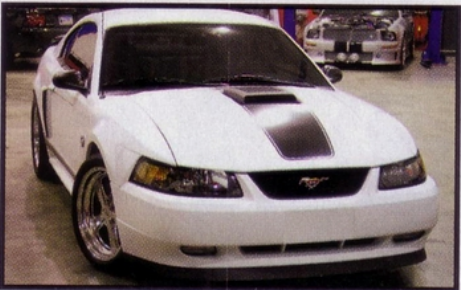
One of Lidio Iacobelli's personal cars is this white '03 Mach 1, which boasts a supercharger, methanol injection and a squirt of nitrous. Apart from cut-down springs to improve the ride height, the suspension is stock. Gearing is 3.73:1. This super-hot street car has run 10.36 off the bottle and as quick as 10.06 on the juice. It looks pretty innocuous for a 10-second street car.
