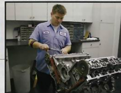
Marc Smielewski is Alternative primary engine builder and assembles the shop's stroker combinations, which take the 4.6-liter short block to a torquey 5.0 liters.
