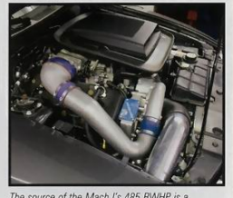
The source of the Mach 1's 485 RWHP is a Vortech-blown and methanol-injected factory four-valve engine.
