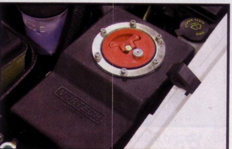
The auxiliary tank under the Mach 1's hood is the methanol reservoir. It enables more aggressive tuning at the track, while drastically reducing exhaust temperature.
