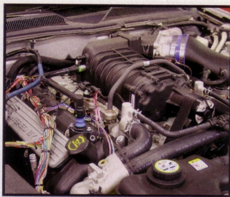
The supercharged 5.4-liter GT500 shoehorned into a GT-based Eleanor clone was dropped off at Alternative Auto to get tuned and running.
