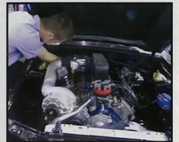
Jay Meisel makes adjustments to a black Fox-body's supercharged, 392-inch Windsor small block. The craftsmanship on the car is outstanding.
