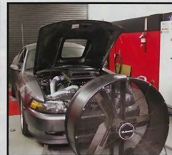
This late-model Mach 1 strapped to Alternative's chassis dyno pumps up 485 horsepower to the tires.
