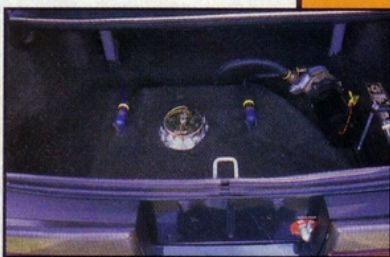
where ice is stuffed in the tank to chill the incoming air charge.
