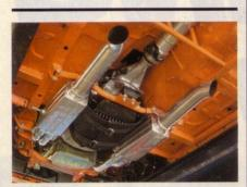
Inside the shrapnel-wrapped 4R70W is a Precision Industries Stallion torque converter, with 5,000-rpm stall. Headers are from Performance Fabrication & Engineering and are vocally restrained by Flowmaster collector mufflers.
