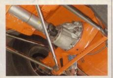
The MPR Racing four-link rear suspension locates a shortened 9-inch stuffed with Mark Williams axles, a spool, and 5.34:1 gears turning huge 15x33 M/T ET Drag slicks. The coilovers are Konis, and the disc brakes are from Lamb.
