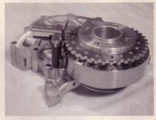
When installed, the damper/trigger wheel assembly will look similar to this. Lidio had to make up metal spacers to properly line up the trigger sensor with the wheel (on the factory Explorer applications, the sensor sat right on the bosses on the timing chain cover, since the trigger wheel was on the backside of the damper).
