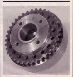
Lidio fits the wheel to an FRPP crank damper (about \$275) and spacer (\$30+/-). To properly reference it with the inductive trigger sensor, the wheel's missing tooth should be aligned with the damper's 30-degree BTDC timing mark.
