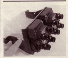
Lidio has so far been able to find used EDIS coil packs, but new ones are about \$90 each from your dealer. The coil pack bracket (\$30) is from the Explorer and bolts right on 5.0s after a bit of grinding to clear a coolant rail. To go on the tallerdeck 351, a little bending and tweaking is needed, but Lidio says it will fit.
