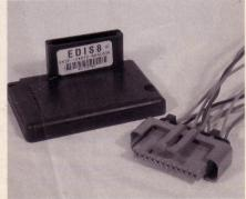
About \$250 will buy you the EDIS8 (eightcylinder) control module and 12-wire harness from a Ford dealer. The module controls firing order, which is common between small-blocks and modulars.
