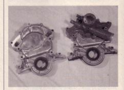
You'll need to buy a timing chain cover that has those two bosses on which to mount the trigger sensor—factory Mustang 5.0 covers did not have them. The version on the right is off the 5.0 Explorer and fits SN-95 applications. The one on the left is for Fox cars (the water pump bolt pattern differs) and is available through Alternative Auto.
