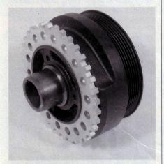
The heart of the EDIS' accuracy is the powdered-metal "36-minus-1"-tooth crank trigger wheel. The only way you can buy it from Ford is as part of this Explorer damper assembly for about \$90. Unfortunately, once you press the wheel off the back, the damper/pulley assembly goes in the garbage as it cannot be used on Mustang applications. Lidio is trying to find a source of the trigger wheel only.
