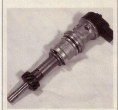
As a distributor replacement plug, use the Explorer 5.0's cam position sensor assembly, which will bolt right into a 302 block (its cam sensor function is not necessary on the bank-fire Speed-Pro; it's just to fill the hole). If yours is a 351-based engine, however, this part will need some modification to fit properly. Lidio can set you up with the correctly modified version.
