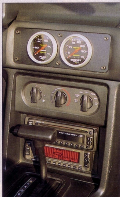
Aaron Treppa monitors the 351's vital statistics with Auto Meter Pro-Comp fuel pressure and boost gauges mounted in the air conditioning vents.
