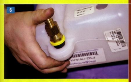
**6.** This fitting feeds the high-pressure pump. All materials have been verified for chemical compatibility when exposed to methanol.
