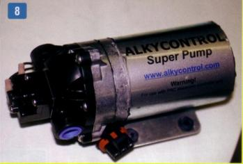
**8.** Here's the big bruiser methanol pump. Don't try and do this with a standard windshield washer pump.
