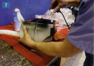
**7.** Being careful to orient the float switch correctly, it goes into the reservoir.
