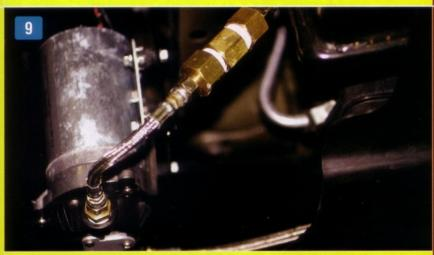
9. The pump gets mounted low on the drivers side of the engine bay along with the associated plumbing.
