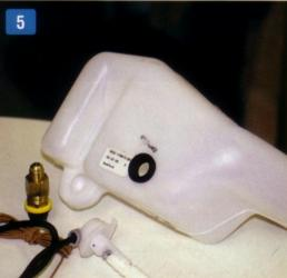
**5.** A modified windshield washer reservoir is used to hold the methanol supply.
