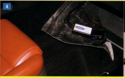
**4.** The injection system's controller and sensitive electronics are kept inside the passenger compartment. Since the system is wired to be active all the time, these modules are mounted behind the passenger's kick panel.
