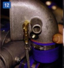
**12.** In Lidio's testing, he found it far better to place the methanol jet in the discharge tube, rather than any earlier in the intake path.
