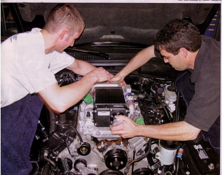
olt-on performance has come a long way since the days of headers and slapper bars. That's especially true of late-model Mustangs, as installing a blower is now little more complicated than swapping an intake manifold.
