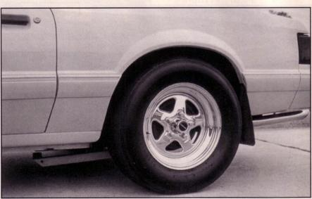
Lakewood traction bars put the power to a factory 8.8 rear carrying 4.10 gears. J60-15 M&H DOT tires were used to put car into the 12.90s with the stock motor. The current 113-mph Vortech combination gets hooked by 28x9 M/T slicks.
