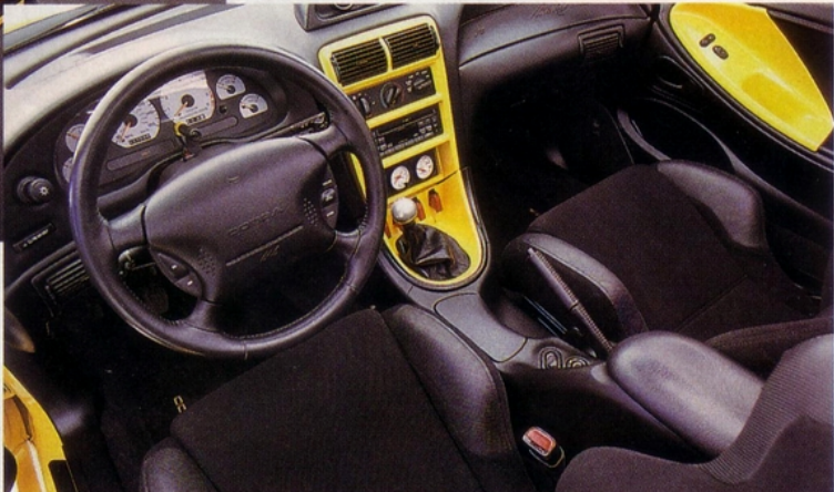
▲ Steve tossed his original seats in favor of these Cobra Daytonas, which come with tracks having far more aft travel adjustment than the legroom-stingy factory setup. These good-looking, supportive buckets, combined with CDC's lightbar and Saleen's Speedster tonneau, really spice up the Cobra's interior.
