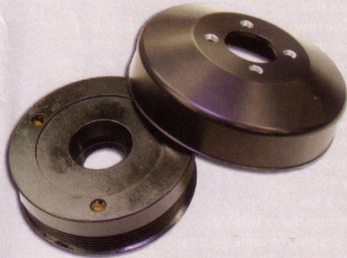
▲ One of the oldest tricks in the Mustang performance book, Lidio bolted up these SFI-approved March crankshaft and water-pump underdrive pulleys. The crank pulley measures 5 inches in diameter, compared to the stock version's 6¼ inches. A stock water-pump pulley is 5½ inches across, while the March replacement measures 6½.
