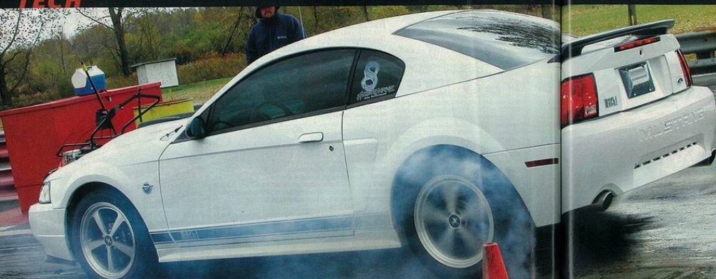
Although most street cars equipped with a Kenne Bell supercharger use the 1700 1.7-liter compressor, Iacobelli decided he needed the extra boost airflow delivered by KB’s larger, 2.2-liter blower. He was looking for the car to make around 600 rwhp. Pump gas is out of the question with the 2200 blower and the Mach 1 engine’s 10:1 compression.
