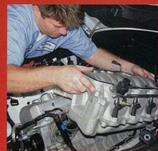
Next, the stock lower intake manifold was removed. Some trimming in the valley was necessary to make room for the blower kit’s intake, but it was comparatively minor surgery.
