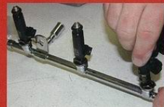
The stock fuel rails were retained but fitted with 60-pound fuel injectors. The car also was upgraded with two in-tank ‘03 Cobra fuel pumps and a Kenne Bell-supplied Boost-A-Pump. The Mach 1 would not lack for fuel.
