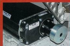
Although most street cars equipped with a Kenne Bell supercharger use the 1700 1.7-liter compressor, Iacobelli decided he needed the extra boost airflow delivered by KB’s larger, 2.2-liter blower. He was looking for the car to make around 600 rwhp. Pump gas is out of the question with the 2200 blower and the Mach 1 engine’s 10:1 compression.
