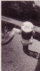
Lidio gutted the stock water pump and replaced its function with this electric unit.
